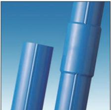
Inclinometer casing is a special tube that used in conjunction with inclinometer probe and characterized by cross shaped groove section along its length. It provides an easy and smooth access for inclinometer probe during subsurface data collection. Inclinometer casing is generally installed in boreholes, however it can also be directly cast inside concrete, embedded in fills or attached to structures. Typically, Inclinometer casing needs to be vertically installed at the center of the borehole.
